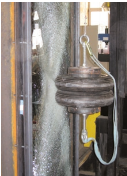
As per standard testing with a drop height of up to 1200 mm
