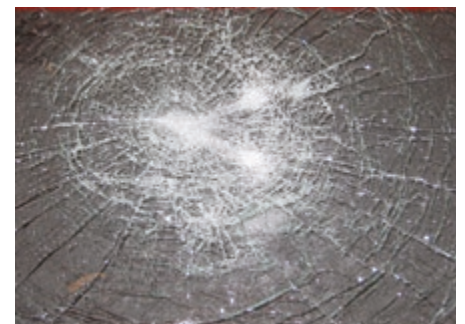
Test passed – no holes in the glass
