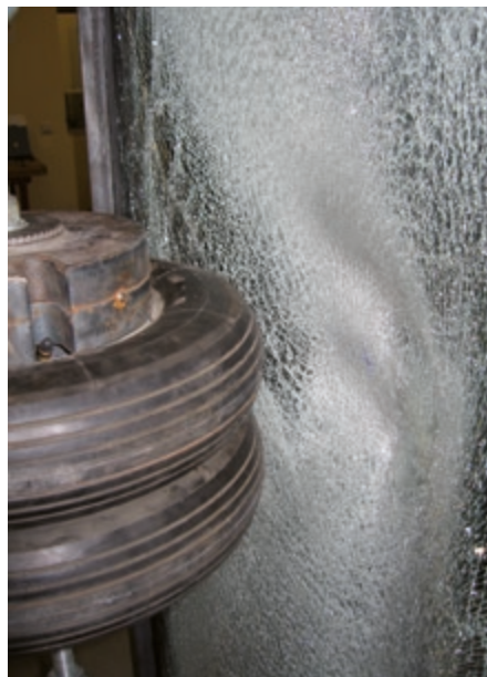
After back swing as per the applicable standard from a height of 100 mm
