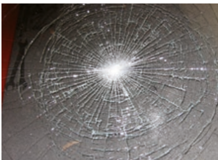
1. Impact from a height of 6 m
